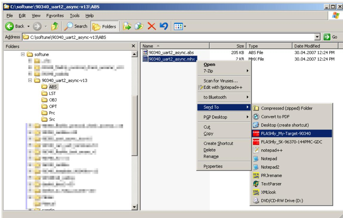
The name of the MHX-file will be added to the predefined parameters and FLASHly will start immediately programming the target application.
